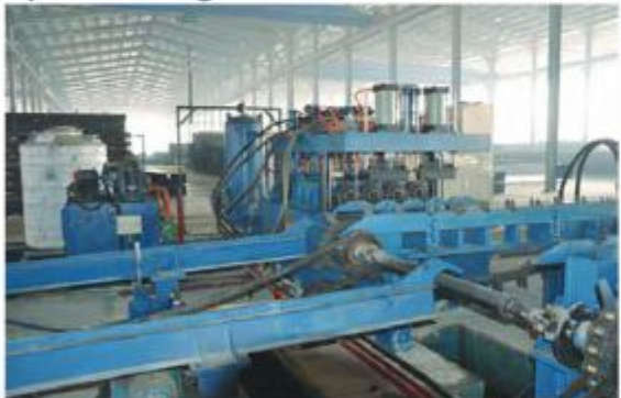
Hydro testing Machines
